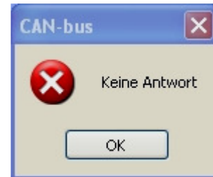
Figure 19: Drive not connected or not switched on, missing terminating resistor
